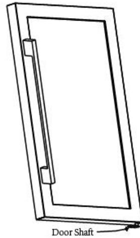
4. Unscrew the screws at the top hinge and lower hinge, and remove the the door hinge. Use a putty knife to prize up the screw hole cover which at the left side of the wine cellar, and re-cover the screw holes on the right side.
