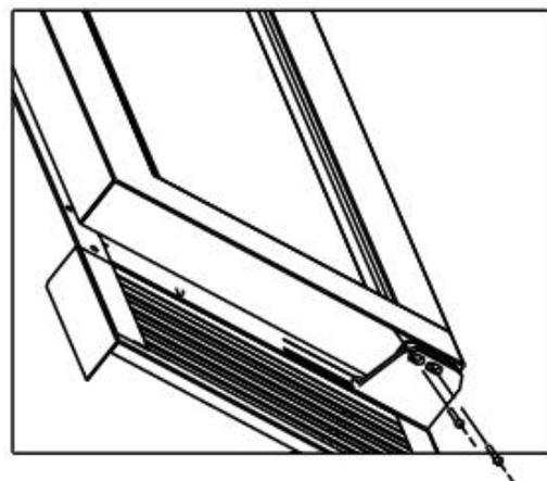
3. Lift the door and take it out from the lower hinge and place it on the mat to avoid damage and scratches. Then remove the adjustable door Shaft.
