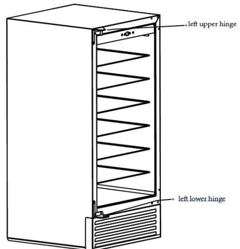
6. Rotate the door 180° , the door should installed the adjustable door shaft first, then relocate the door to the designed position.
